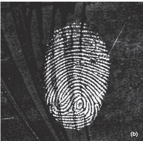
FIG. 5—Ethyl cyanoacrylate fumed fingerprint on Coke aluminum drink can: (a) White light photograph, (b) Monochrome representation of FTIR chemical image.
